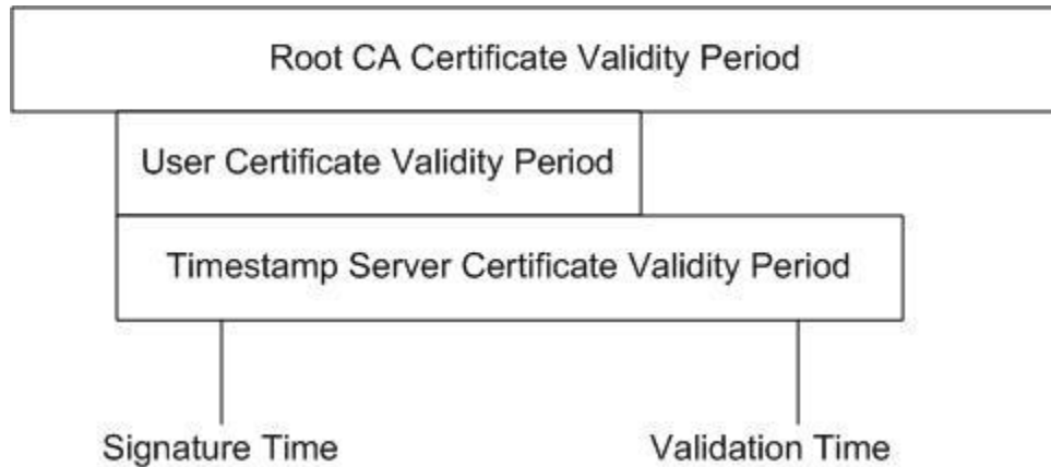
Figure – Validating a signature when the timestamp is valid, but the signature certificate is expired. The expiration of the signature certificate does not matter, because the authoritative timestamp indicates a time when the certificate was valid.
